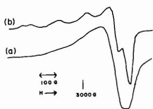
Fig. 3. ESR spectrum of complex 4a at 77 K, (a): pH 9.7, (b): pH 5.4.
